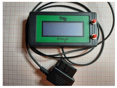
The on-board computer is designed to help you diagnose problems with the Td5 engine. An additional advantage is the possibility of continuous monitoring engine parameters while driving.
